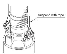
Operate the pump in a location that has a sufficient water level and collects water easily.
