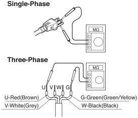
**Note:** The insulation resistance reference value of 20M  $\Omega$  minimum is based on a new or repaired pump. For reference values of a pump that has already been put into operation, refer to "7. Maintenance and Inspection" of this manual.
